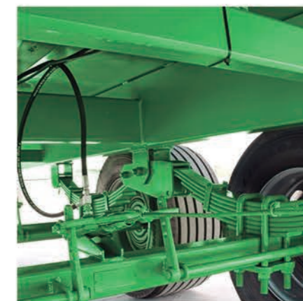
BALLESTA MULTIHOJA Y ABARCONES REFORZADOS/ MULTILEAVES SPRING AND REINFORCED U-BOLTS
