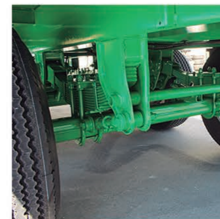
BALLESTA MULTIHOJA Y ABARCONES REFORZADOS/ MULTILEAVES SPRING AND REINFORCED U-BOLTS
