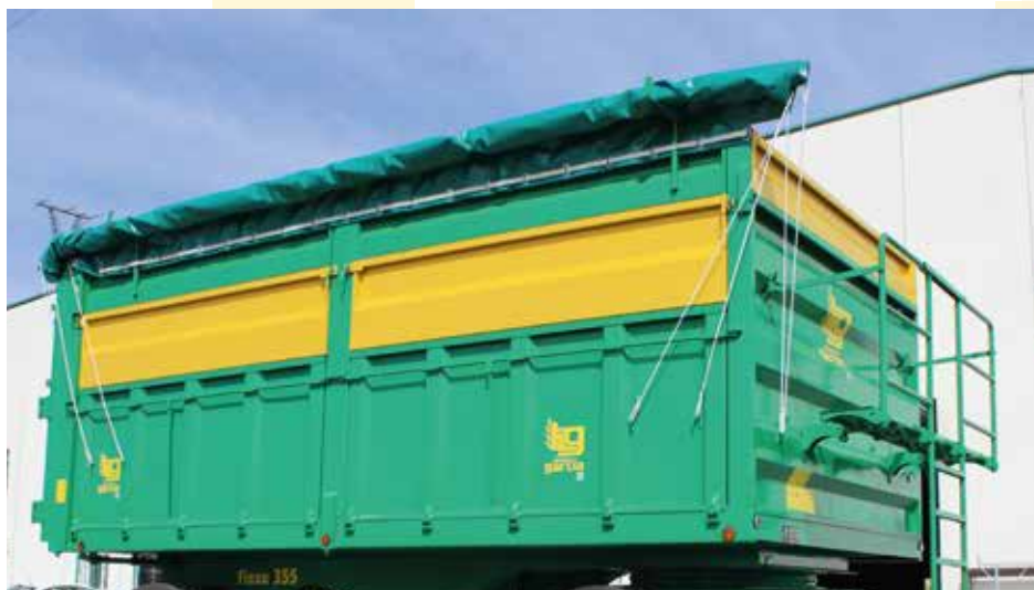
• Lona de barra lateral con balcón plegable Lateral canvas bar with folding balcony
