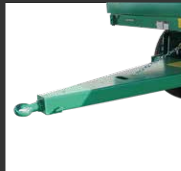
Anilla soldada welded ring
