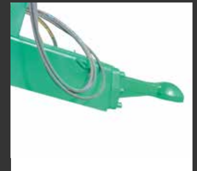
Bola atornillada screwed ball
