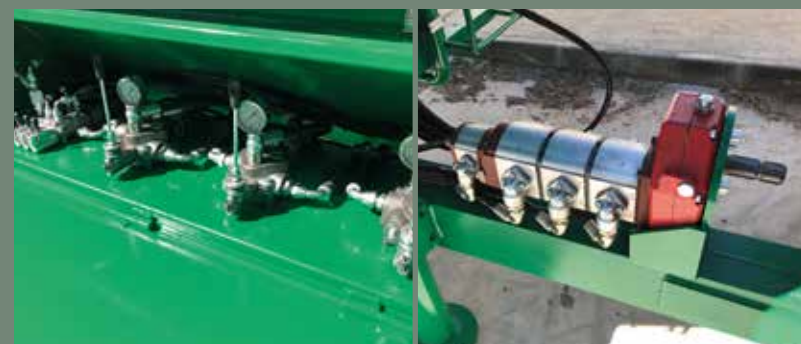
Bombas y mandos hidráulicos / Hydraulic pumps and controls
