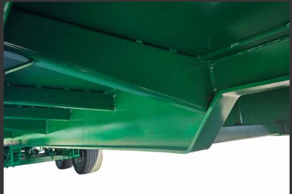
Acero ST52 120x12-6 ST52 steel 120x12-6
