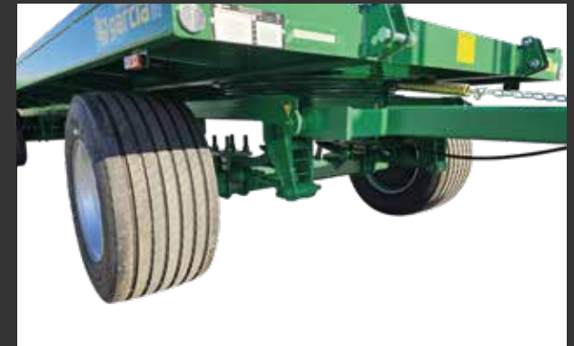
1º eje ballestas con tensores (3-4 ejes) 1st axle with leaf springs and tensioners (3-4 axles)
