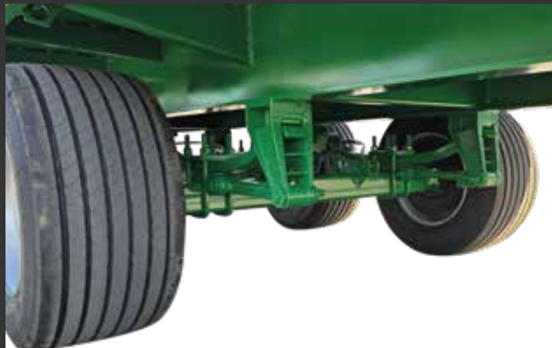
4 ballestas tándem tensores 4 tandem leaf springs with tensioners
